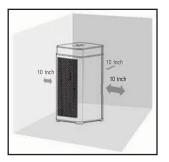
Do not obstruct the air intake or the clean air outlet. To ensure proper air circulation, leave at least 10" space between the back air intake and the wall or the furniture.
