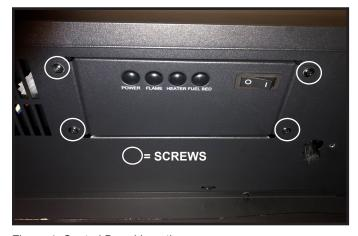
Figure 4 Control Board Location
