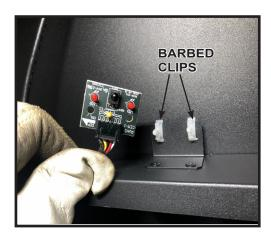
Figure 13 Receiver Removal
