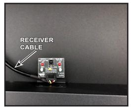
Figure 12 Receiver Location and Cable
