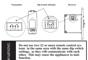
Do not use two (2) or more remote control systems in the same area with the same dip switch settings, as they will communicate with each other. This may cause the appliances to malfunction.
