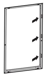
After determining the left or right hinge position, secure with the four field supplied mounting screws. The Access panel frame must be plumb (vertical) and level.
