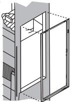
For a left hand hinge mount the door frame with the three hinge tabs on the left side.
