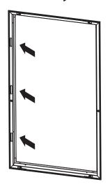
For a right hand hinge mount the door frame with the three hinge tabs on the right side.
