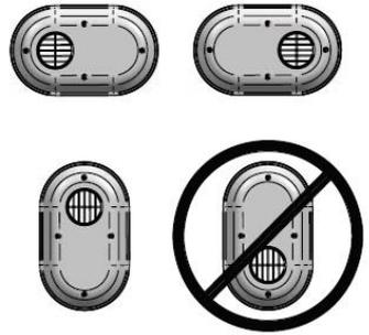
**Figure 3 – Approved Installation Orientation**
