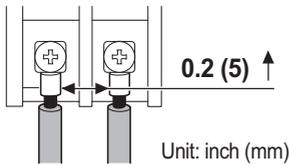
※ The distance between wires should be more than 0.2 inches (5 mm).
