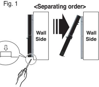
**Remove remote controller by inserting a screw-driver into the lower separating holes and twisting to release the controller from backplate.**
