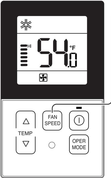
**1** Select the proper fan speed which you want by pressing the
