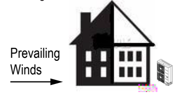
Figure 54: Leeward Side of the Building.
