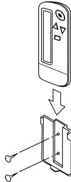
2. Slide the remote controller (2) into the remote controller holder (3) from the top.
