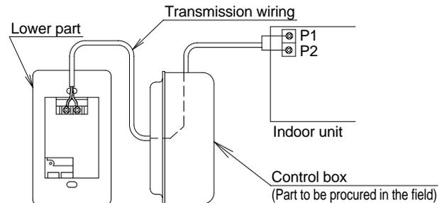
(Connect the P1 and P2 terminals on the rear of the lower part to the P1 and P2 terminals on the indoor unit. Neither of the terminals is polarized, so it is not important if connections are crossed.)
