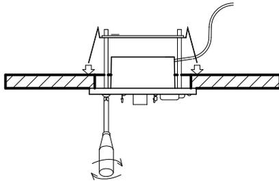
(Tighten both screws (8) evenly. Overtightening may deform the case and possibly make it harder to install the upper part.)
