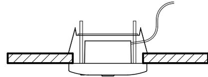
(Install the upper part on the lower part being careful parts are facing in the correct direction. After installation, turn on the power, and test emergency run button.)
