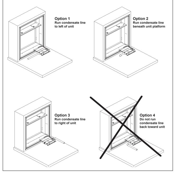
IMPORTANT - The drain pan and line must be kept free from debris. Prior to installing the chassis ensure that there are no blockages in the drain pan or line.
